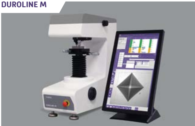
Vickers/Knoop Micro-Hardness Tester Force range: 0.01 kgf to 1 kgf [Deadweight]
