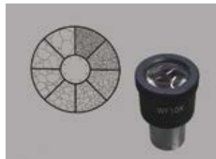
Eyepiece, WF 10x, with ASTM Grain Size E112
